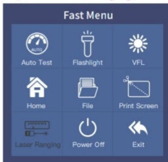
Press the "≡" icon at the bottom of the screen to enter the quick operation menu, and press different function icons to enter the corresponding function interface or realize the corresponding operation functions.
