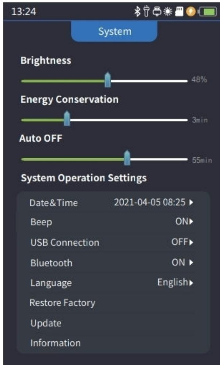
**Brightness:** slide the progress bar to adjust the backlight brightness
