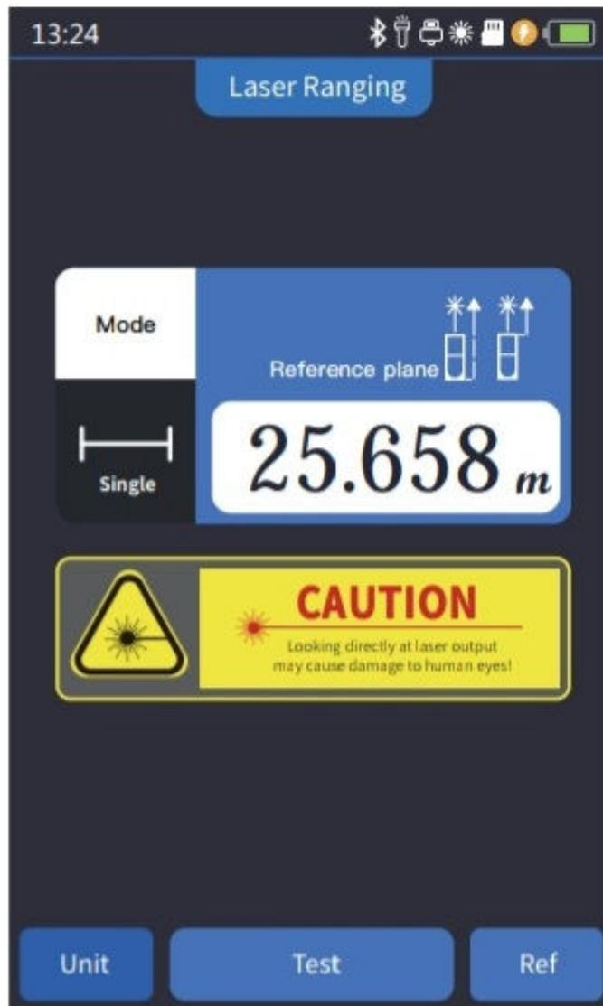
**Laser Range:** the maximum test distance is 40 meters
