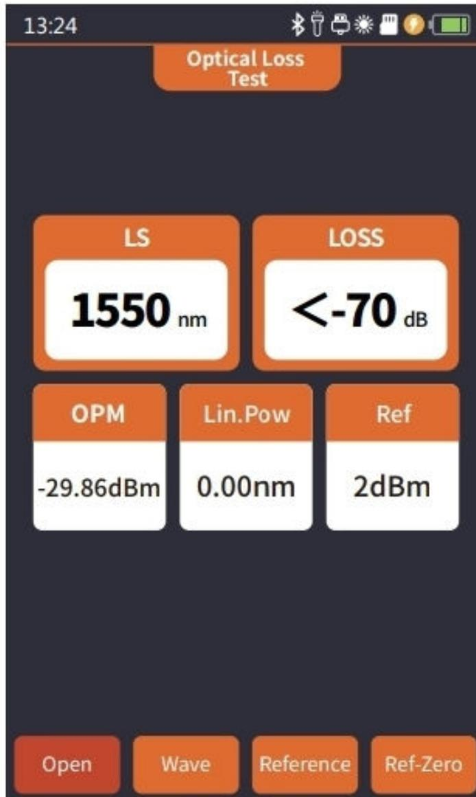
**Used to test the insertion loss of optical passive components.**
