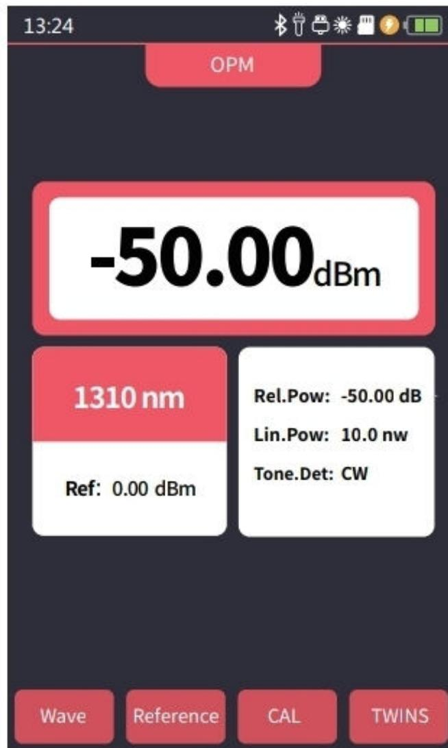
The function is used to test the power of optical signal and insertion loss of various devices and optoelectronic components. It can identify and measure the frequency of 270/330/1000/2000Hz optical signal.
