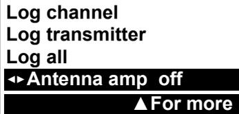
The HD-T2 features an on board DC supply of 5 Volts for active antennas and 12 Volts for mast head amplifiers. This feature makes it easier to install amplified antennas as a cable does not need to be run to provide the 5 or 12 Volts during antenna installation. With the Antenna amp option highlighted select the voltage required by using the right or left arrow button.
