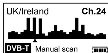
The real-time histogram will enable you to select a channel number of interest. Depending on the mode selected the display in the lower left corner will reflect this choice and also indicate a lock. By selecting the On button you can view the measurement values directly.
