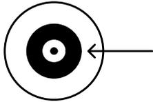
**Tip:** Check for any copper fragments that may have gathered in the well of the F barrel socket on the meter. These can be removed with a dry cotton bud or air duster. When replacing with a new F barrel connector avoid over tightening, it should only be tight enough to prevent removal by hand.
