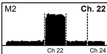
Selecting the Spectrum (wide) function will show a wider span so that more adjacent carriers are visible.
