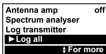
Log all will scan from the bottom of VHF to the top of UHF logging any carriers that are found above the squelch threshold.
