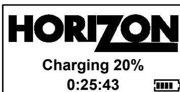
During battery charging the LCD will be active but not back lit, and the current percentage of charge will be shown along with the duration of time that the meter has been on charge. During charging the battery icon in the lower right of the display will animate.
