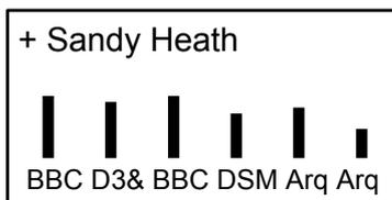
On selecting the standard the next screen of the slope test shows a histogram of the levels of each mux available from the previously selected transmitter. This is especially useful for the installation of distribution systems. Pressing the right arrow button again will show the slope comparison.
