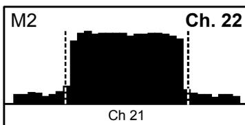
Selecting Spectrum (channel) will display the channel of interest in the centre of the display window. Press the left or right arrow buttons to navigate up or down frequency. Press the On button to exit to the measurement mode or the OK button to return to the primary sub menu.
