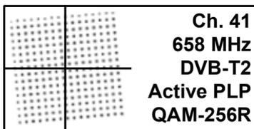
Shown here on the left is a QAM-256 Rotated constellation. To zoom in on the constellation diagram use the On button to select different regions of the diagram. QAM and QPSK constellations are supported. You can return to the measurement mode by pressing the Off button once.
