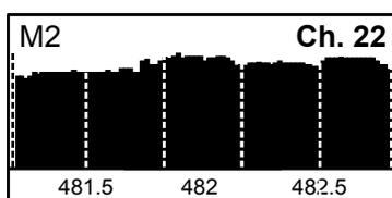
Selecting the Spectrum (narrow) function will fill the display with a narrow span of the selected channel.
