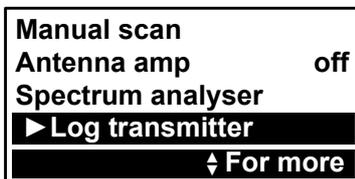
The Log transmitter function will group log all of the available services from the selected transmitter in an incremental fashion where the leading number remains constant and the number after the dash increments.
