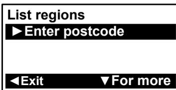
The HD-T2 features a useful transmitter lookup by post code feature this enables you to enter the first half of the installation site post code and you will be presented with a list of transmitters to choose from for that region. **Note:** The transmitter selections marked with a plus symbol are the power transmitters.
