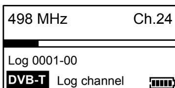
Here we can see that the measurement values of channel 24 are being logged to entry 0001-00.
