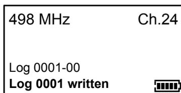
Once the log has been written you can press the **OK** button to return to the measurement mode, alternatively the meter will return to measurement mode after a few seconds.
