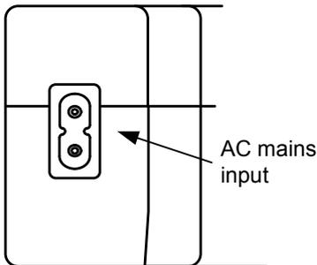
For AC charging a suitable figure of eight mains lead is supplied. The charge circuit can operate on AC voltages from 90 to 250V
