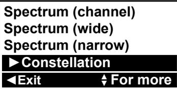
The constellation diagram function is only available once a lock has been obtained on a DVB-T/T2 mux and is available from the primary sub menu by pressing the OK button during the measurement mode.
