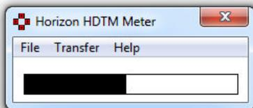
Open your received file and a small program will appear as illustrated above. If you have already connected your meter to your computer and downloaded the drivers you can click on **Transfer** to load your new transmitter settings into your meter. The driver installation is detailed on the next few pages.
