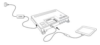
The tablet/smartphone automatically activate the application recognizing the programmable amplifier model.
